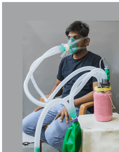
reBreather: Breathing device to enhance lifetime of O_2 cylinders
