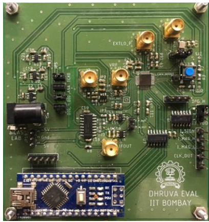
Dhruva: Indian RF receiver chip for NAVIC & GPS Satellites
