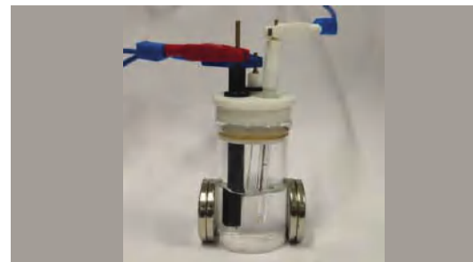
Energy-efficient hydrogen production using magnetised catalyst
